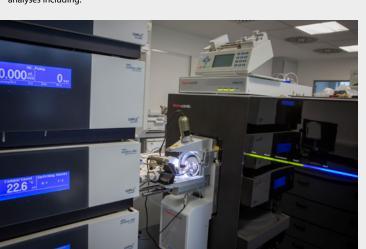
which was installed at the end of 2019, has far superior performance in terms of scan speed, sensitivity and resolution, and has some additional capabilities (including FAIMS interface, high mass-range, and UVPD fragmentation). This enhanced performance will enable us to analyse complex, low abundance samples in much greater detail, which is essential in trying to identify critical regulators of important biological processes, and to understand how they function.
